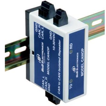
The CAN is connected to the system through terminal blocks. A power supply of 10-30 VDC is required. Model CANOP is housed in a rugged DIN-rail mountable box, making it easy to install in an industrial cabinet.
