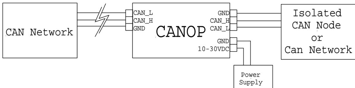
The CAN network must be terminated at both ends according to the CAN specification. Networks not properly terminated may have data errors, or miss the data completely. The CANOP creates two new ends to the CAN network. Space is provided on the board for a termination resistor on each side, R6 and R8. A 120-ohm resistor is recommended for the termination. If the CANOP is not at the end of the network, it should not be terminated.
